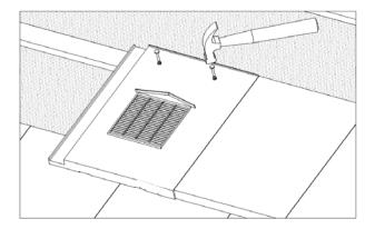
3 - Place the throat of the ventilator through the underlay aperture and ensure that all moulded interlocks and integral clips are engaged with the adjacent tiles before nailing the ventilator in place.
