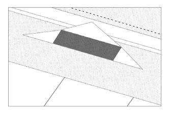
2 - Ensure that the top and lower flaps of the underlay are on the upper surface of the underlay just above the batten. Cut a 340mm long slot in the underlay to accept the underlay protector which should pass under the batten and into the slot. This needs to be done prior to locating the ventilator.
