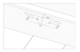
1 - Determine the position for the ventilator between rafters. Just below the batten, cut and fold the underlay as shown to accept the throat of the ventilator. Ensure that cuts in the underlay do not extend beyond the sides of the throat.
