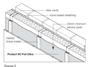
Timber frame construction. Foil side facing into the service void airspace.
