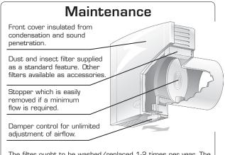
The filter ought to be washed/replaced 1-2 times per year. The Standard filter is washable (use a gentle detergent). The Pollen and Environmental filter should be replaced with a new one. The filter is placed in the front cover, which is easily removed.
