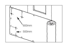
2. Secure membrane to sheathing with austenitic stainless steel staples at 500mm centres vertically and 600mm horizontally
