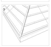
3. Screw fix hip batten constructed from 50 x 50mm timber to the supports.
