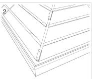
2. Hip batten supports in 50mm x 50mm timber should be screw fixed at the eaves and apex and spaced along the line of the hip rafter in between the tiling batten spaces as shown. Supports could be constructed from 2 x 25mm tiling battens.
